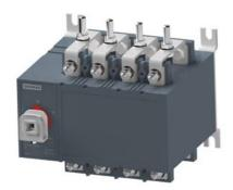
SINOVA, onload changeover switches 3KJ1, manually operated, size 1, 4-pole, in open execution, Iu: 100 A, Ue AC: 415 V, le at AC-22 A at 415 V: 100 A, screw mounting, front operating mechanism, at the left end, complete unit with door operating mechanism, Plastic handle, grey and black colour, flat terminal
