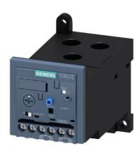
Overload relay 12.5...50 A Electronic For motor protection Size S2, Class 10E Stand-alone installation Main circuit: Straight-through transformer Auxiliary circuit: Screw Manual-Automatic-Reset
