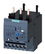
Overload relay 10...40 A Electronic For motor protection Size S0, Class 5...30 Contactor mounting Main circuit: Screw Auxiliary circuit: Screw Manual-Automatic-Reset Internal ground fault detection
