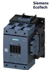
power contactor, AC-3e/AC-3 115 A, 55 kW / 400 V, AC (50-60 Hz) / DC Uc: 220-240 V 3-pole, auxiliary contacts 2 NO + 2 NC drive: conventional main circuit: box terminal control and auxiliary circuit: screw terminal
