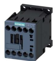
power contactor, AC-3e/AC-3, 7 A, 3 kW / 400 V, 3-pole, 24 V DC, auxiliary contacts: 1 NO, screw terminal, size: S00
