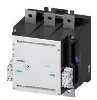
vacuum contactor AC-3e 630 A, 335 kW / 400 V, AC-3 820 A, 450 kW / 400 V, Ue 690 V, 3-pole, Uc: 110-132 V AC(50/60 Hz) drive: conventional auxiliary contacts 4 NO + 4 NC main circuit: busbar control and auxiliary circuit: screw terminal
