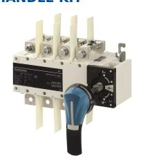
between two sources for any low voltage power circuit, as well as safety isolation with double breaking per pole. In addition to source changeover function, they can as well be used for source inversion (e.g. to change the direction of a motor) or grounding/earthing. They are availlable in 3 or 4 poles.
