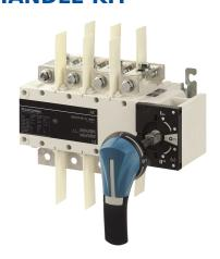
between two sources for any low voltage power circuit, as well as safety isolation with double breaking per pole. In addition to source changeover function, they can as well be used for source inversion (e.g. to change the direction of a motor) or grounding/earthing. They are available in 3 or 4 poles.
