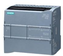
SIPLUS S7-1200 CPU 1214C DC/DC/DC based on 6ES7214-1AG40-0XB0 with conformal coating, -20...+60 °C, compact CPU, DC/DC/DC, onboard I/O: 14 DI 24 V DC 10 DQ 24 V DC 2 AI 0-10 V DC, power supply: DC 20.4-28.8 V DC, program/data memory 100 KB
