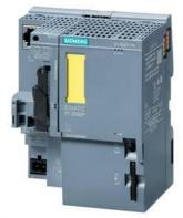
SIPLUS ET 200SP CPU 1512SP F-1 PN based on 6ES7512-1SK01-0AB0 with conformal coating, -25...+60 °C, central processing unit with work memory 300 KB for program and 1 MB for data, 1st interface, PROFINET IRT with 3-port switch, 48 ns bit performance, SIMATIC Memory Card required, BusAdapter required for port 1 and 2
