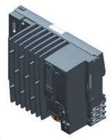
SIPLUS ET 200SP CPU 1515SP PC2 L based on 6ES7677-2DB40-0GB0 with conformal coating, -40...+60 °C, 8 GB RAM, 128 GB CFast, Ready4Linux, S7-1500 software controller CPU 1505SP preinstalled, interfaces: 1x slot CFast, 1x slot SD/MMC, 1x connection for ET 200SP BusAdapter PROFINET, 1x 10/100/1000 Mbps Ethernet 2x USB 3.0; 2x USB 2.0, 1x DisplayPort, documentation on USB flash drive,
