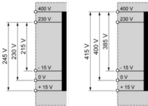
Secondary Voltage Wiring
