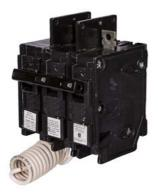
Siemens Low Voltage Molded Case Circuit Breakers General Purpose MCCBs - Type BQ, 2-Pole, 120/240VAC are Circuit Protection Molded Case Circuit Breakers. 2-Pole Common-Trip circuit breaker type BQ. Rated 120/240V (015A) (AIR 10 kA). Special features: 120VAC Shunt Trip. Note: Load side lugs are included.
