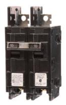
Siemens Low Voltage Molded Case Circuit Breakers General Purpose MCCBs - Type BQ, 2-Pole, 120/240VAC are Circuit Protection Molded Case Circuit Breakers. 2-Pole Common-Trip circuit breaker type BQH. Rated 120/240V (015A) (AIR 22 kA). Special features: Load side lugs are included.
