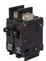
Siemens Low Voltage Molded Case Circuit Breakers General Purpose MCCBs -Type BQ, 2-Pole, 120/240VAC are Circuit Protection Molded Case Circuit Breakers. 2-Pole Common-Trip circuit breaker type BQH. Rated 120/240V (080A) (AIR 22 kA). Special features: Load side lugs are included.
