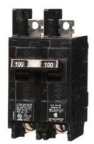
Siemens Low Voltage Molded Case Circuit Breakers General Purpose MCCBs - Type BQ, 2-Pole, 120/240VAC are Circuit Protection Molded Case Circuit Breakers. 2-Pole Common-Trip circuit breaker type BQH. Rated 120/240V (100 A) (AIR 22 kA). Special features: Load side lugs are included.
