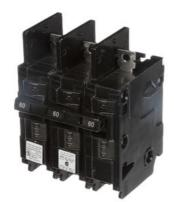
Siemens Low Voltage Molded Case Circuit Breakers General Purpose MCCBs are Circuit Protection Molded Case Circuit Breakers. 3-Pole Common-Trip circuit breaker type BQH. Rated 240V (060A) (AIR 22 kA). Special features: Load side lugs are included.
