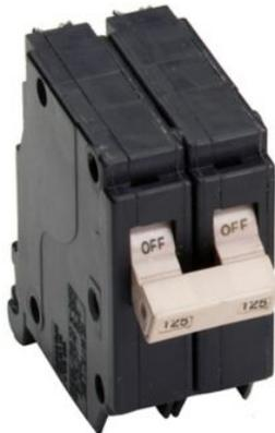
Eaton CH Thermal magnetic circuit breaker, Type CH 3/4-Inch standard circuit breaker, 125 A, 10 kAIC, Two-pole, 120/240V, CH, Common breaker trip, #10-1/0 AWG Cu/Al, CH, Type CH Loadcenters
