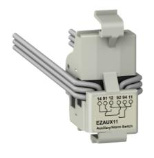
auxiliary and alarm switch AL AX, EasyPact EZC 100, EasyPact CVS 100BS, 2 common point changeover contacts
