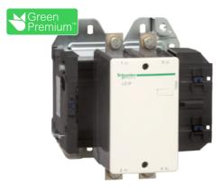
TeSys F contactor - 2P(2 NO)-AC-1 <= 440V 700A with coil LX1/ LX9 - 48...1000V AC 40/400Hz, LX4 -48...440V DC
