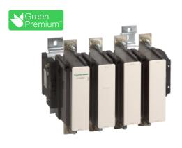
TeSys F contactor - 4P(4 NO)-AC-1 <= 440V 1000A with coil LX1/ LX9 - 48...1000V AC 40/400Hz, LX4 -48...440V DC
