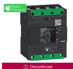
circuit breaker ComPact NSXm E (16 kA at 415 VAC), 4P 3d, 80 A rating TMD trip unit, compression lugs and busbar connectors
