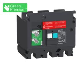
Earth-leakage VigiPacT add-on protection module, ComPacT NSX 250, 200VAC to 440VAC, 30mA to 30A, 3 poles
