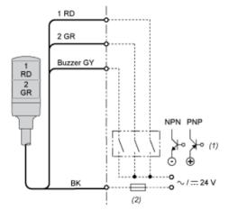
"ON" for lighting and/or applying continuous sound. Fuse (rated current: 0.5 A)
