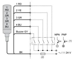
"ON" for lighting and/or applying continuous sound. Fuse (rated current: 0.5 A)
