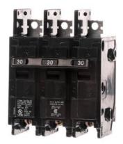
Siemens Low Voltage Molded Case Circuit Breakers General Purpose MCCBs are Circuit Protection Molded Case Circuit Breakers. 3-Pole Common-Trip circuit breaker type BQ. Rated 240 V (030A) (AIR 10 kA). Special features: Load side lugs are included.
